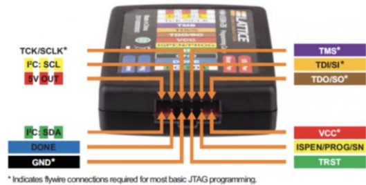
* Indicates flywire connections required for most basic JTAG programming.
