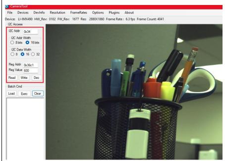
Register access function: This camera supports register access function. The I2C address is 0x34 To the left is an example: 0x36c0, 0x36c1 is the exposure register address.
