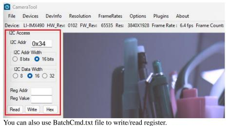
Register access function: This camera supports register access function. The I2C address is 0x34
