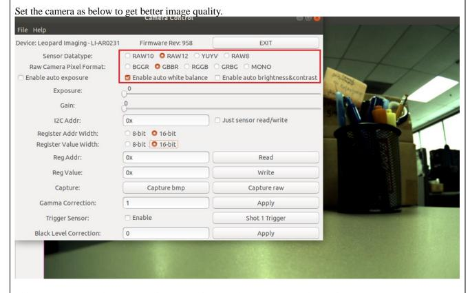
This camera tool can be used to write/read registers and capture Raw and BMP images.
