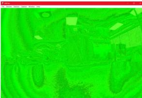
Note: This camera tool supports Raw-to-RGB function which will reduce the display frame rate. You can click Options → DisableDisplay to get actual frame rate from the sensor. You can also use other regular software (like AMcap) to get higher frame rate, but the video will be green (like below) due to lack of Raw-to-RGB conversion function.
