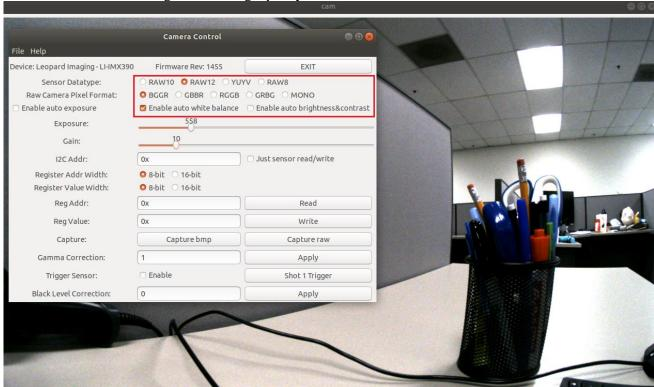
This camera tool can be used to write/read registers and capture Raw and BMP images.
