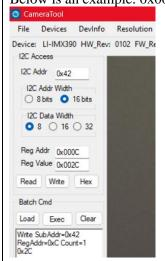
You can also use BatchCmd.txt file to write/read register.
