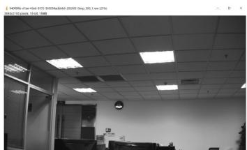
Note: This camera tool supports Raw-to-RGB function which will reduce the display frame rate. You can click Options  $\rightarrow$  DisableDisplay to get actual frame rate from the sensor. You can also use other regular software (like AMcap) to get higher frame rate, but the video will be green (like below) due to lack of Raw-to-RGB conversion function.
