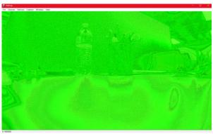
Note: This camera tool supports Raw-to-RGB function which will reduce the display frame rate. You can click Options → DisableDisplay to get actual frame rate from the sensor. You can also use other regular software (like AMcap) to get higher frame rate, but the video will be green (like below) due to lack of Raw-to-RGB conversion function.
