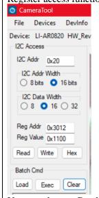
This camera supports register access function. The I2C address is **0x20**
