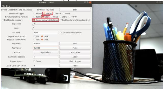
This camera tool can be used to write/read registers and capture Raw and BMP images.
